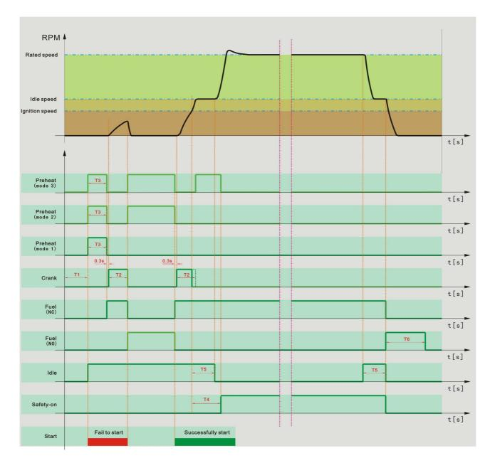
T1 - start delay T4-safety-on delay
